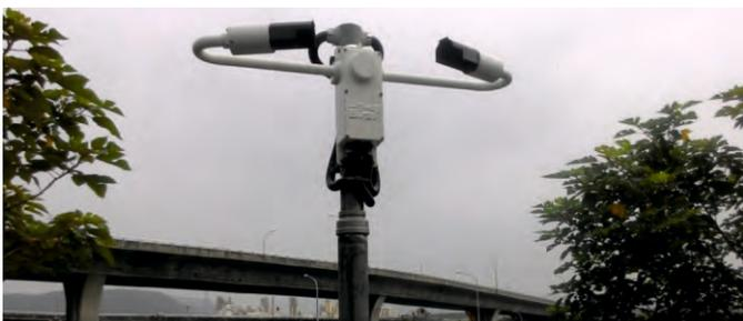
RS232, RS422 or RS485 interface. The standard data message provides averaged MOR however the user can select an EXCO output if preferred. The only option available for the SWS-050 is an interface to the ALS-2 Ambient Light Sensor for use in aviation applications where RVR information is required. The ALS-2 Ambient Light Sensor data is appended to the standard sensor data message simplifying both the installation and data processing.
